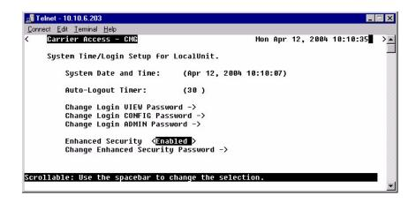
When Telneting into the Router with Enhanced Security enabled, the following will appear:
